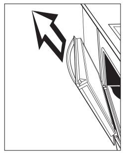
■ Lift the door upwards until it rests partially open, as shown, then lift upwards to remove. In this position the hinges are prevented from closing.
